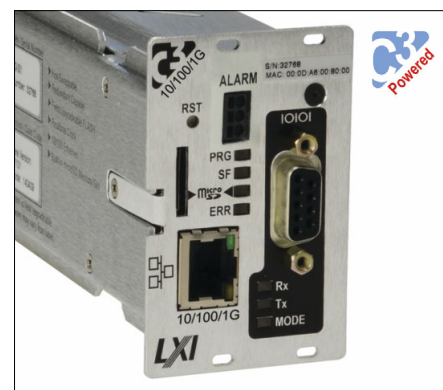
Plug-in C3 and C3-Lite Controllers certified LXI with TCP/IP, HTTPS (SSL/TLS), SNMP v1/v2C/v3, SNTp, IPv4/6 and REST. Latest in hot-swap control interface technology with the best in network security layers and protocols, plus fast 10/100/1GB hardware with auto-negotiation.
