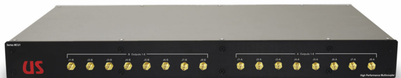
Example: MCU1-D8NRAF34 Unit has two sections of 1x8, inputs on the rear via N-Type connectors, outputs on front via SMA, +3dB gain and frequency range "4" (see table above).
